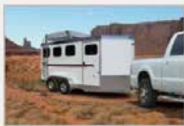
Nomad BP Aluminum slant load bumper pull horse trailer with wedge nose.
