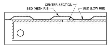
Figure G1: Cut away view of bed and center section.
