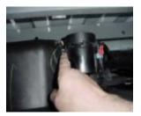
Figure C2, Step 2: Disengage the locking pin.
