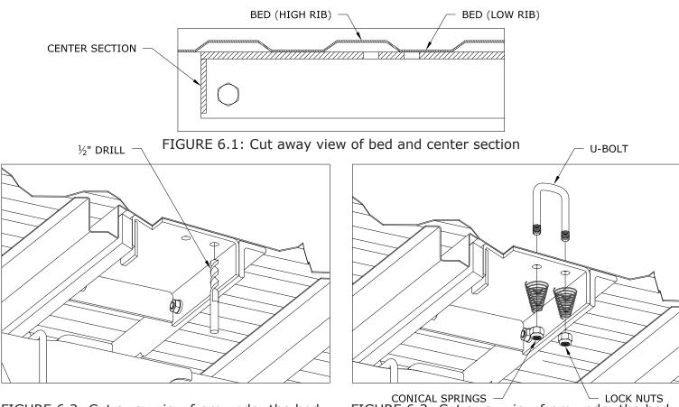
FIGURE 6.2: Cut away view from under the bed
