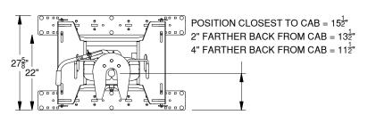
TABLE A2: Distance from edge of rear rail to pivot point. (Rails, Base and Coupler shown fully assembled)
