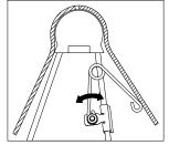
Figure E2: Cutaway view of driver pivot arm and saddle.
