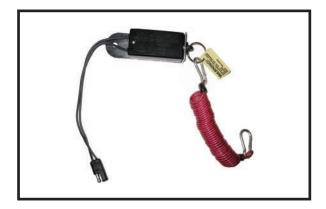
**BRK2505:** There is one (1) breakaway switch included with your Patriot 3<sup>®</sup>. An additional switch for a second vehicle can be purchased.
