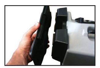
**BRK2503:** The seat stiffener works with any drop in tow brake on the market. It provides a larger surface area on the seat for the brake system to push against. This means you get better, more responsive braking.
