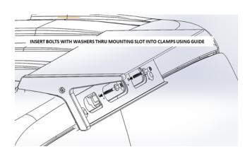
8. Final Securing of the Platform: BE SURE TO CENTER AND LEVEL THE PLATFORM ON THE VEHICLE CAB. Holding the Platform Assembly firmly against the vehicle, tighten the clamp adjustment fasteners to take up the slack until the gaskets fit uniformly against the profile of the cab body and compress the leading edge deflector gasket. Sight the top of the endcaps as a reference for level and true. Final tighten both clamp fasteners equally to flatten the lock washers, 15-18 ft/lbs each.
