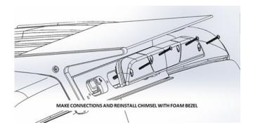
Connect the new apparatus' wiring harnesses and test. Add the provided foam bezel, reconnect the CHMSL harness, and reinstall light housing into Platform Assembly with original fasteners.
