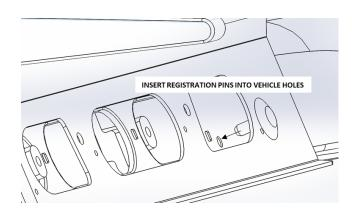
7. Installation of the Platform: Pull all harness wires and CHMSL lead though the access holes. Insert mounting bolts with washers thru the platform mounting hole and align with clamp registration grommet. Carefully adjust the location of the clamps to maximize hole alignment and thread bolt in loosely.
