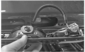
**2.** Unplug the wire harness connector(s) and set Light assembly aside. **3.** With the 3rd Brake Light Assembly set aside, remove the factory plastic screw anchors (Fig. 2) and secure the supplied two Retainer Plates into the opening using provided hardware as shown on Fig. 3, 4. Tighten #10-32 nuts (4 pcs.) firmly against the truck's frame.
