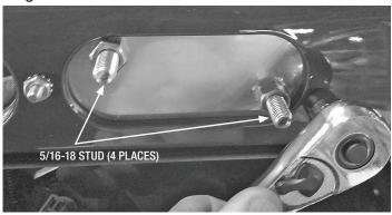
**4.** Inspect the gasket of the Mount and mating surface of the truck to ensure that surface is free of any defects or foreign materials.
