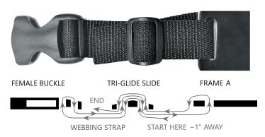
**9.** Assemble Male Buckle half (item 12) to Triglide (item 14) and to Tension Lock (item 13) using the other 16" Webbing Strap (item 11) as shown in the figure. Carefully note the position of the Tension Lock. The ribbed bar should be facing up.
