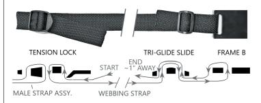
**11.** Assemble two Trigluides (item 14) to frame location C on Base (Item 1) using the 30" Webbing Strap (item 11) as shown in the figure. Using the Triglide, create approximately a 3" loop at the end of the strap assembly.
