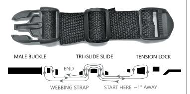
**10.** Assemble the strap assembly created in step 9 to Triglide (item 14) and to frame location B on Slider Arm (item 3) using the 20" Webbing Strap (item 11) as shown in the figure.
