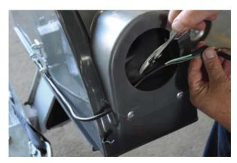
14. Pull all wire from light hole in housing and install the snapper hose clip approximately 1-1/2" back from end of wire shielding. Squeeze snapper clip tight with pliers.
