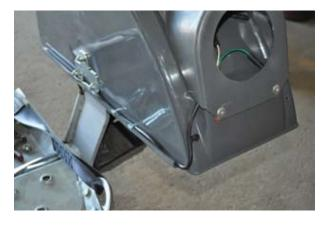
15. Push wires back into housing and finish routing wires in wire trough of fender and attach cable hanger. With pliers install two metal wire clips. Place one clip 5-1/2" from rear of fender and one 8" from rear of fender.
