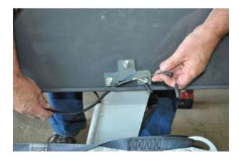
12. Fish the three wires from the mainframe through the front hole in the fender trough.
