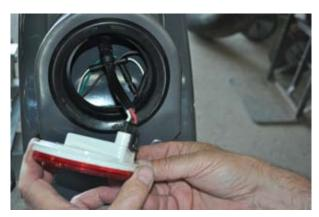
Install rubber grommet and attach 3-wire pigtail harness to fender wiring. Coil pigtail harness inside of fender housing and plug into 4" round LED light. Push light into grommet.
