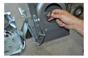
13. Route wiring in through back of tail light housing on the bottom inside of housing. Fish the three wire inside of housing.
