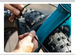
Position the wheel strap to be centered on the bike's rear wheel. Insert the strap into the latch as shown. Adjust the wheel strap sleeve (#6) over the wheel and pull the strap firmly through the latch.
