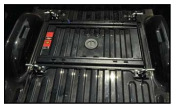
4. Pull back on main frame towards back of truck and snug bolts. Make sure sockets are free to operate and main frame can be easily removed. Once this is done torque all bolts to 35 ft-lbs. NOTE: Locking sockets are in the locking position in picture. Once bolts are checked once again make sure frame can be removed and operate properly.
