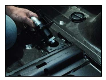
2. Place front locking sockets (silver locking tabs) into main frame and lock. Insert four 3/8" x 1.00" flanged head bolts to each socket and leave loose. Reference front drawing for direction of locking sockets.
