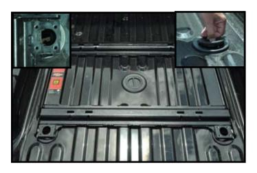
1. Remove covers from each mounting pod and place main frame into box of truck over mounting pods as shown.
