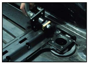
**3.** Place rear locking sockets (gold locking tabs) into main frame and lock. Insert four 3/8" x 1.00" flanged head bolts to each socket and leave loose. Reference front drawing for direction of locking sockets.
