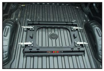
1. To fit the frame for the truck pods, remove covers from each mounting pod and with the locking arm bolts loose enough to move the locking mounts, place main frame into box of truck over mounting pods so the locking arms fit into the truck pods as shown.
