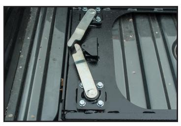
**3.** Once your latches are setup for your truck, turn handle in so they will lock into each other as shown in picture.
