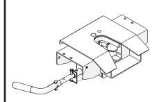
To uncouple, remove saftey pin, pull handle straight out until the jaw locks open. If jaw will not stay open, install safety pin in second handle hole just outside of frame handle bushing.
