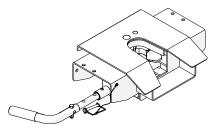
Remove safety lock pin if installed and pull handle until jaw locks open.
