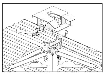
5. Install 5th wheel head with the 1" pin.
