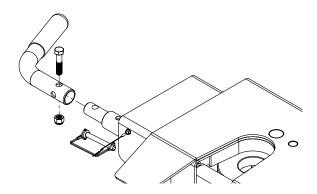
**Note (Read carefully before installing):** Handle can be positioned toward the front or the back if it is found to interfere with the trailer in any way. Verify this before traveling.
