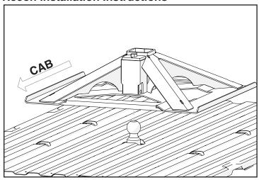
Place Recon base over gooseneck 2-5/16" ball so ball fits into the recon ball coupler. NOTE: Ball coupler socket goes towards cab of truck.
