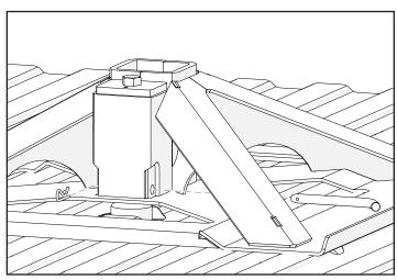
2. Slide coupler pin into coupler hole, making sure pin goes under gooseneck ball. Top coupler bolt may need to be lossened for pin to go under the ball.
