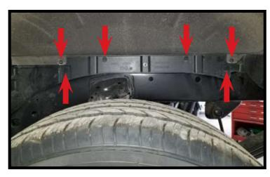
**3.** Remove plastic filler panel by removing four plastic push fasteners and two screws.
