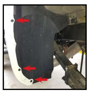
**4.** Remove plastic wheel well filler panels by removing three screws.
