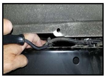
**5.** On the drivers side of the vehicle, remove two plastic clips from the frame.
