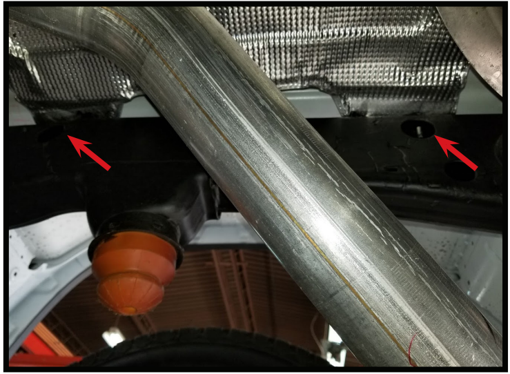
Inside of frame: The other access holes are on the inside of frame. These holes are located right behind the bracket. No trimming is need, but you may have to move some steel lines out of the way to fish the bolts through.
