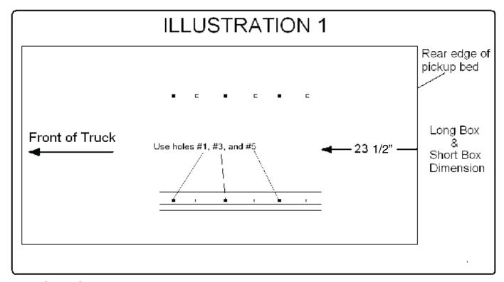
**CAUTION:** Do not install base rails over plastic bed liners. Plastic bed liners must be
