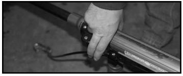
**Step 2.** Use the latch trigger handle to release the connecting legs between the two vehicles by pressing down on the latch trigger handle. One connecting leg may have more pressure against it, do that one first.
