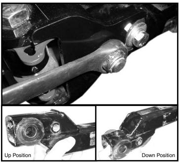
**NOTE:** The Dominator comes with a 1-1/2" off-set receiver that can be flipped to help level the tow bar with the towed vehicle. The receiver is in the up position from factory, to change to the lower position, remove both 1/2" bolts and washer from side of receiver joint head. Remove the 3/4" nut and bolt, slide receiver out of receiver joint head and flip receiver into the down position. Slide receiver back into the receiver joint head and reinstall the fasteners.
