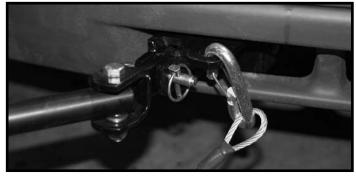
**Step 5.** Slide and twist the legs into position to attach them to the baseplate on towed vehicle. Secure to baseplate using the two attaching pins and 1/4" quick-lock pin. Attach safety cables (see below). Now connect the lighting cable between the towing vehicle and the towed vehicle lighting system or optional light bar. The coiled section of the cable will be stored on the support rod. Towing vehicle must be larger and at least 500 lbs. heavier than the towed vehicle and tow bar combined.
