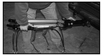
Step 2. Insert the Dominator into a Class III or IV hitch.
