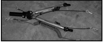
**Step 1.** Out of the box, the Dominator tow bar is setup for the recommended positions for the safety cables and light wire storage rod. These can be positioned to new areas to fit your setup by loosening the screw on the retaining rings and sliding them off the rail and relocating to a new position and tighten screw. Install the light cable (optional) by placing the coil over the wire support rod. Secure the cable with the cable locking hair pin.
