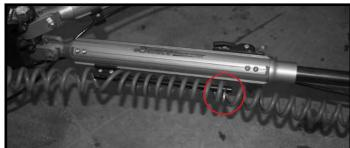
**Step 7.** Leave the electrical cable storage pin (circled above) out for the locking procedure in step 6. When step 6 is completed, position cable on storage rod leaving enough slack, and insert pin.
