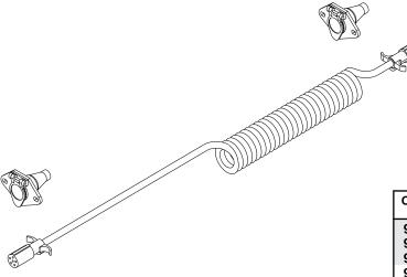
NOTE: To be used with optional Light Bar, the ends will have to be cut off light bar harness. This end will then need to be wired to the receptacle of the auxiliary lighting kit.
