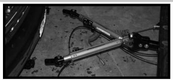
**Step 4.** Position the vehicle to be towed approx.24" behind the towing vehicle. Perform a tow bar safety check, look for any loose fasteners, condition of safety cables, excessive movement in connecting leg shaft when the shaft is extended and locked. If any excessive movement or loose fasteners, the tow bar will need to be serviced before towing. The vehicles **do not** have to be in straight alignment to complete the hook-up. **Engage towed vehicle and towing vehicle parking brake.**
