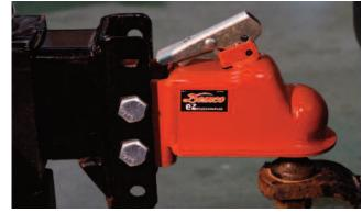
(2) At the mid-way point when lowering the trailer, the stem on the handle will begin to rise up allowing the ball to enter the ball socket.
