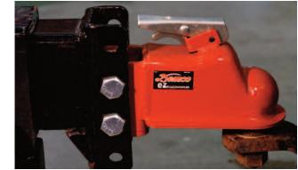
(3) Once the ball has fully engaged the socket the ball keeper will snap back into place securing the coupler to the ball.
