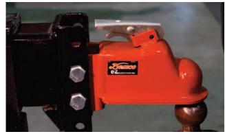
(1) eZ-Latch couplers do not require users to lift the handle for the coupler to engage the ball. Position the ball in the center of the ball socket or slightly forward, then begin to lower the coupler with the jack on the trailer.
