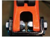
(4) 5/8" Grade 5 Bolts are required with channel mounted 2" & 2 5/16" couplers
