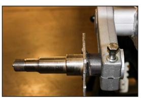
11. Thread the bolt into the torsion arm and tighten to 120 **Ft. Lbs**.
