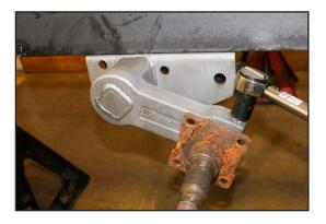
4. Using a thin, steel wedge, tap the wedge into the slot at the rear end of the torsion arm. This will expand the arm socket slightly and release the clamping pressure holding the old spindle in place.
