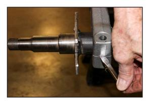
10. Use only the ½"-20 bolt included in the spindle replacement kit (bolt has adhesive thread locker already applied).
