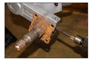
5. Keep the wedge in place and pull the old spindle from the socket. You may need to use a slide hammer to dis-lodge the spindle if access to the back side is not possible.
