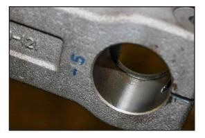
7. With the wedge still in place, insert the new spindle. Rotate the spindle as needed to align the flat surface to engage the mating flat surface inside the socket.
