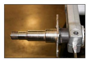
9. Remove the wedge and insert the ½"-20 clamp bolt (with lock washer installed) in from the top side of the torsion arm.
