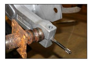
6. With the spindle removed from the socket, carefully clean out any remaining debris. Apply a light coat of rust preventative to the inside surface of the socket.
