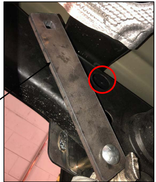
Figure 9: Passenger Side Rear Use the larger top hole shown above for fishing Carriage bolt (7) and block (8).
