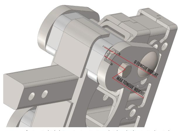
After Being Used Multiple Times, Zero Point May Have to be Relocated Without Any Weight on Hitch (Simply unscrew set screw & relocate to zero point & retighten).
