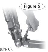
Attach the tow bar arm to the quick-disconnect base with one of the included base pins (Figure 6). Attach the arm so that the head of the shoulder bolt (Figure 6) is facing up. Lock the base pin with a linch pin (Figure 6) or optional padlock – part number 301 (one padlock) or 302 (two padlocks).
