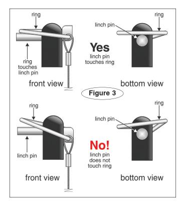
Failure to properly attach and lock all linch pins will result in the loss of the towed vehicle, which may cause property damage, personal injury or even death.
