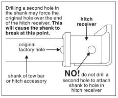
weaken the steel. The shank may break during towing, which will cause the towed vehicle to separate.
