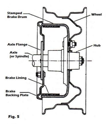
(Section view showing relationship of typical wheel, hub, stamped drum, and brake on axle)
