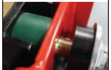
Figure 5: Main frame touching bushing - stop adding air
