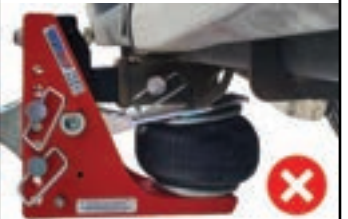
Figure 2: Excessive angle - spacer recommended
