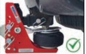
Figure 1: Good angle - no spacer needed
