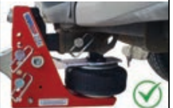
Figure 3: Excessive angle fixed with spacer block
