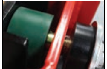
Figure 4: Main frame not touching big bushing - add air
