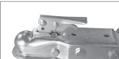
Coupler Locking Mechanism Closed - Figure 4-4
